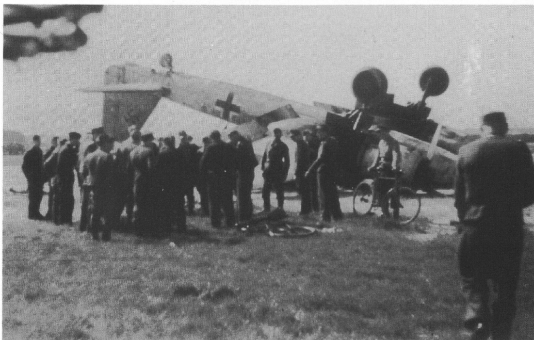
Left: The Mistel combination resulted in an unfavorable center of gravity, so that even Schulmisteln had an "allergic reaction" to rough spots on the runway. Flip-overs such as these were the results.
