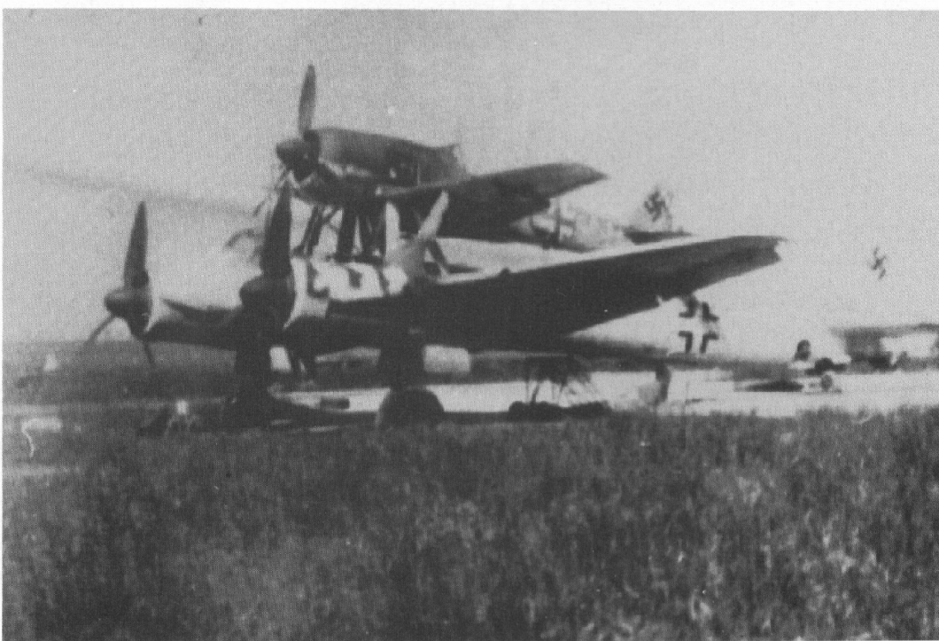
This Schulmistel most probably never went into operation. Based on the paint scheme, the lower component was actually planned for night missions.
