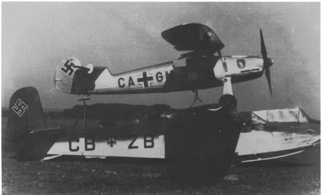
Above: Fw 56 "Stösser" as the control aircraft. Note the clearly discernible rope pyramid and the wheel supports on the DFS 230.
