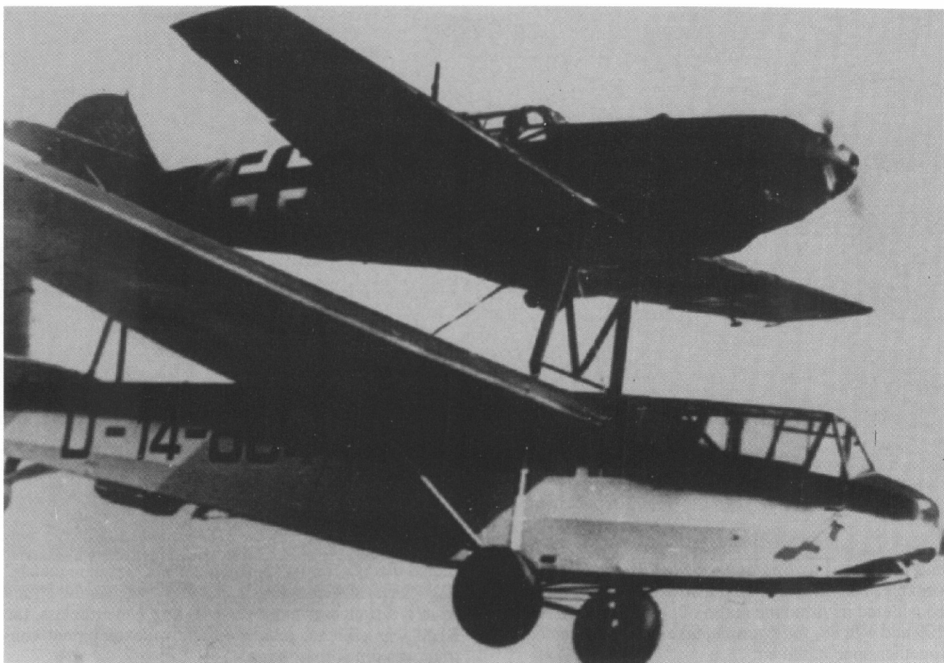
Bf 109/DFS 230 with a simple brace. For comparison, the lower photos show the version with dive braking mechanism.
